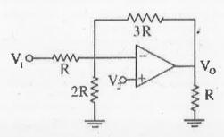
(ii) For given circuit the operational amplifiers are ideal find out the output voltage Vo. (5)
